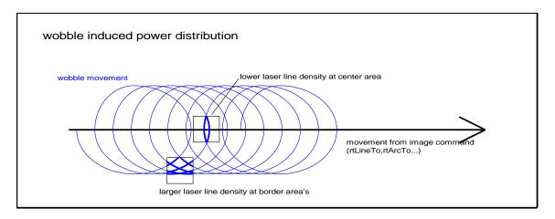
Wobbling is automatically switched off when the laser goes inactive to minimize power consumption. After configuration, the application can suspend or change wobble direction and phase between vector lines by using the function *rtSetWobbleMode*
