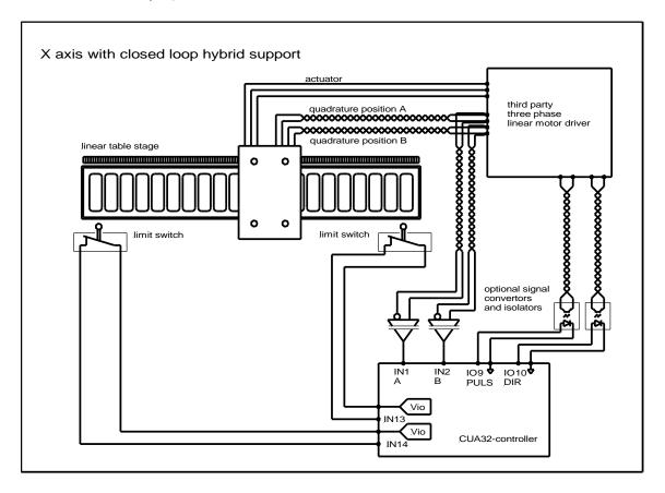
When image processing should be done using both deflectors and stages the resolver input and hybrid marking can be switched on and parameterized. This implementation is called closed loop hybrid marking because the CUA32-controller uses the measured actual position as input. This closed loop hybrid solution comprises more wiring but is likely to have a higher accuracy.
