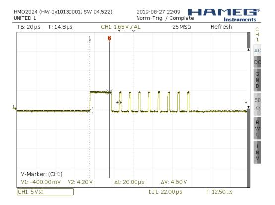
The first pulse measured when this script was run equals 22  $\mu$ sec. This results from the concatenation of the 20  $\mu$ sec wake up pulse with the first burst pulse.
