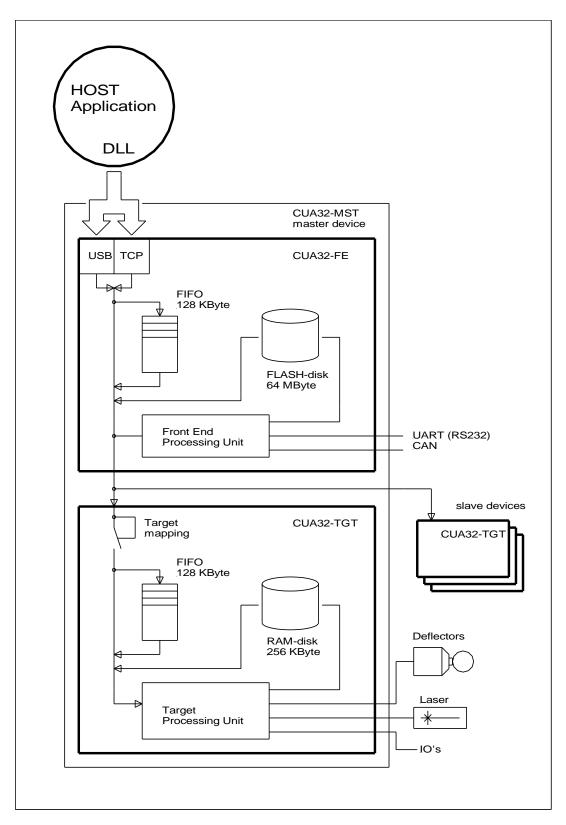
The CUA32 device is connected to the host computer over USB or ethernet. Data flow over this connection is managed by a DLL (rhothor.dll) comprising a large set of functions to query and command the CUA32 system. Queued functions are executed on a fifo based system while
