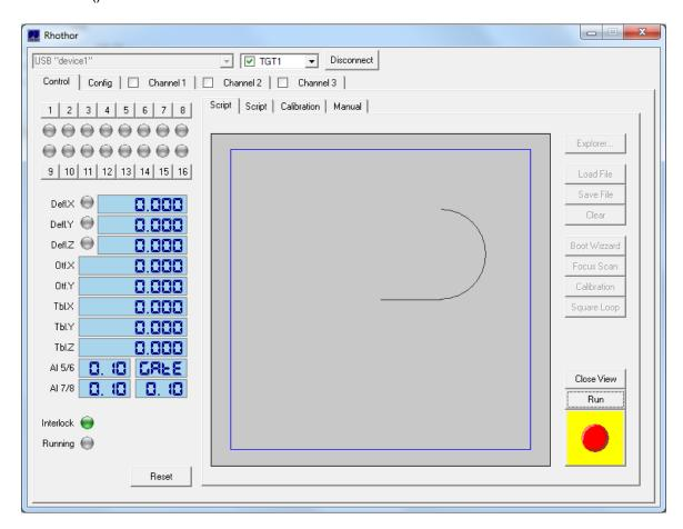
After the example code was loaded into the script editor, the rhothor executable simulates the marking by pressing the View button. The arcs center point lies at (20,15) and runs counter clockwise over an angle of 180 degrees. (*BF* = tangent(45°))
