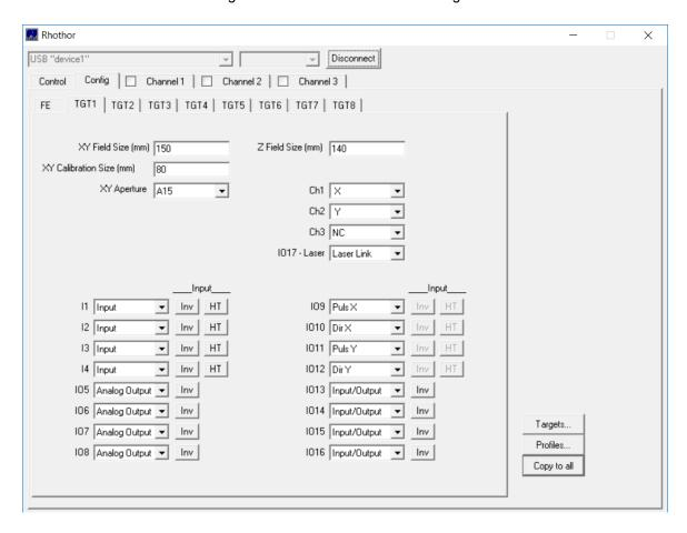
This configuration only allocates the IO pins. Before a table axis can be used, following data needs to initialized:
