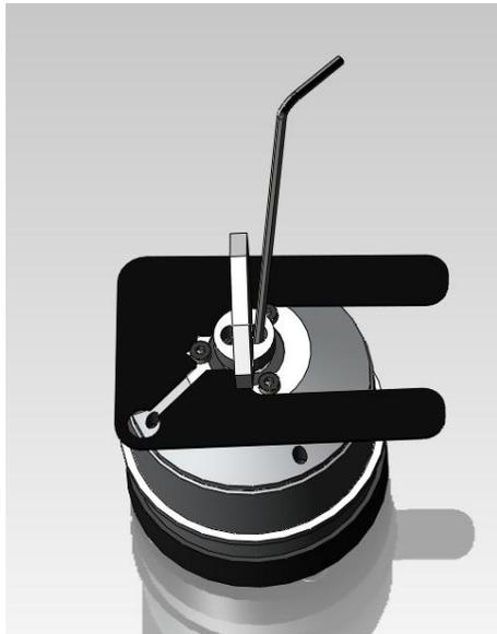
While pressing the alignment tool around the mirror holder, softly tighten the mirror locking screws without putting force on the motor itself. When too much force is given on the motor, the controller card will turn off the motors.
