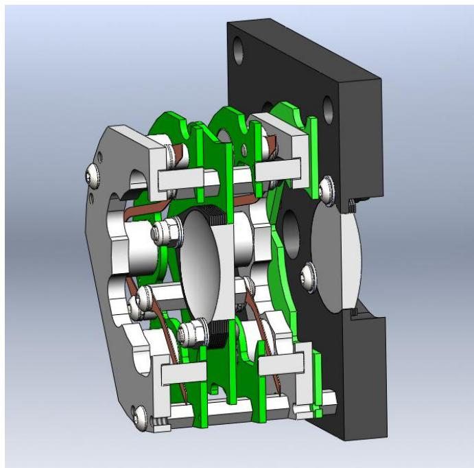
Use special studs to secure the spring bearing before exchanging the lenses.
