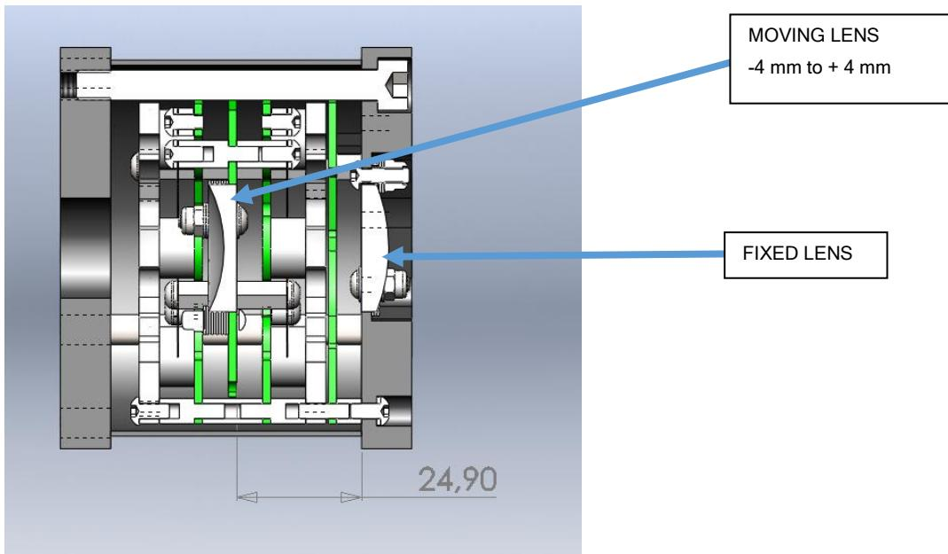
Inside the focus shifter the lens reference planes are 24.9 mm apart from each other when the focus shifter is regulating in 0 position. Depending on the desired lens combination - lenses can be mounted with spacers to get a desired distance between moving and fixed lens.
