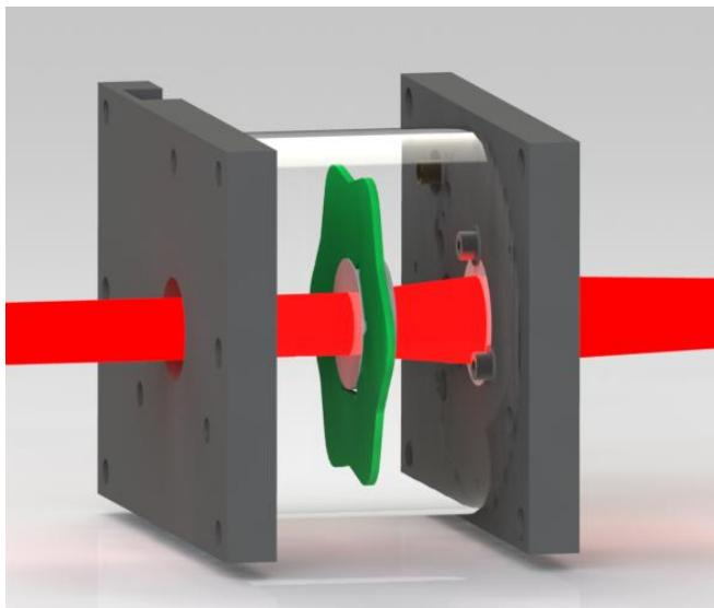
By mechanically shifting the negative focal length lens the output beam divergence will vary.
