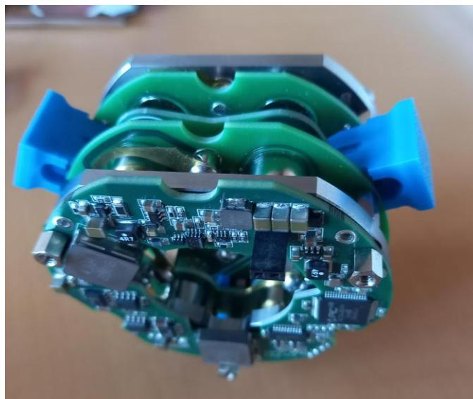
The PCB for the moving lens includes threaded holes for M3 screw. M3x10mm screws are pre-mounted. The lens itself is held in place by dedicated lens fixtures and secured using nylon washers.
