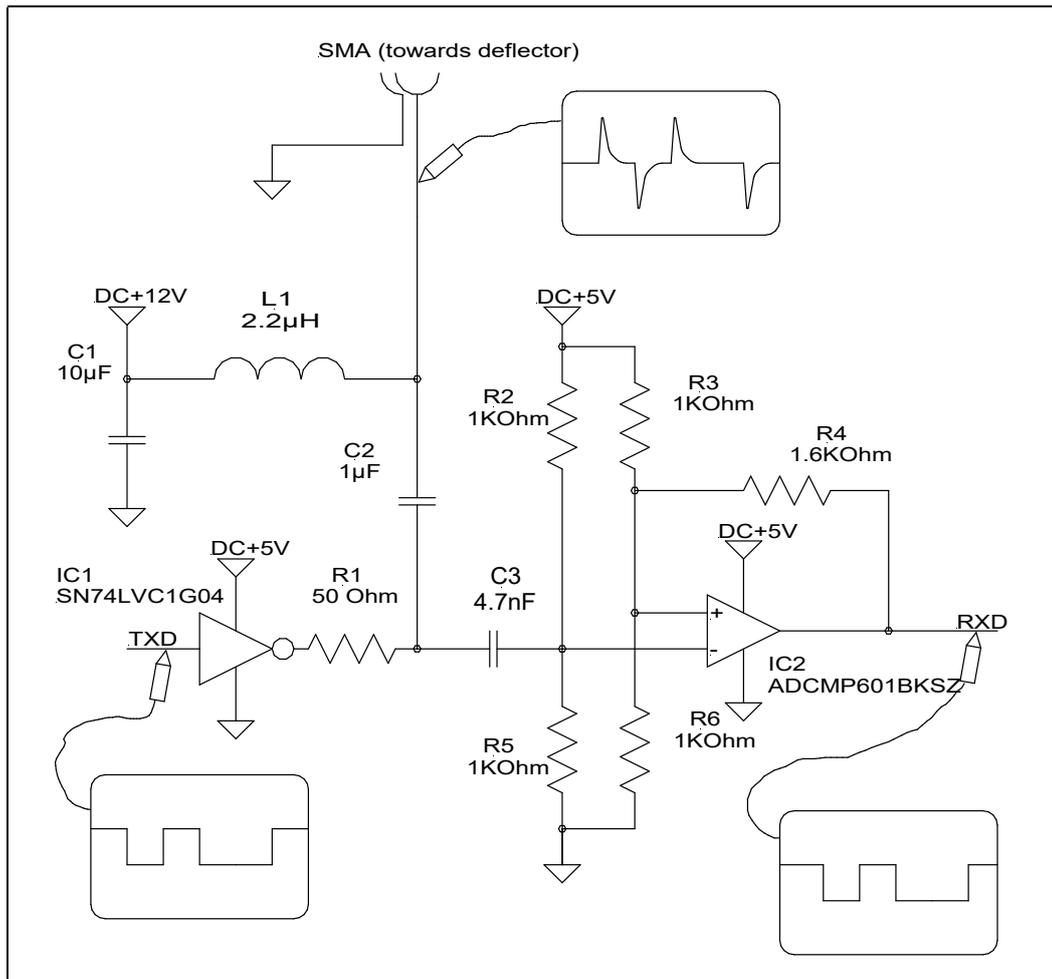
The data towards the deflector (TXD) is high pass filtered while the power supply (DC+12V) is low pass filtered. The high pass filtering is achieved through inductor L1 and resistor R1. Capacitor C2 only serves as a DC level shifter between output amplifier (IC1) and the deflector's power supply. The time constant of the high pass filter equals 44 nsec ( $2.2\mu\text{H}/50\Omega$ ). The saturation current of inductor L1 should be high enough to handle the deflector's peak currents.
